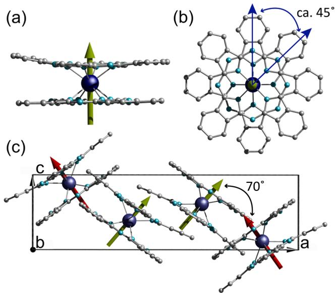
FIG. 1. Molecular structure and packing of  $[\text{TbPc}_2]^0$ : (a) side view; (b) top view; and (c) packing diagram of the molecules in the  $Pnma$  unit cell, displaying two magnetically inequivalent sets of molecules with their easy axes (red/green arrows) tilted approximately  $70^\circ$  with respect to each other. Color scheme: Tb, purple; N, blue; C, gray; H atoms have been omitted for clarity.
